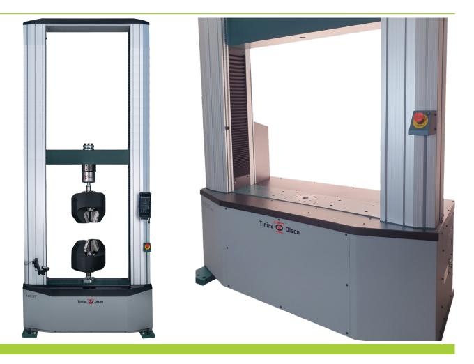
The 100ST Extended height & width model is an Electromechanical Materials Testing Machine. It is a robust design for use in a range of materials testing.
