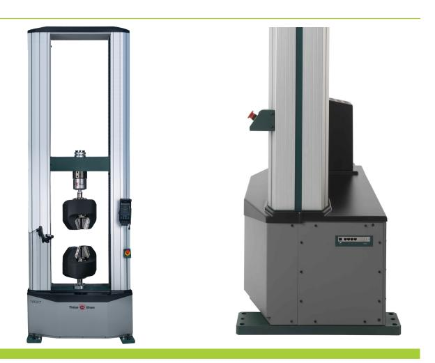
The 100ST Extended height model is an Electromechanical Materials Testing Machine. It is a robust design for use in a range of materials testing.
