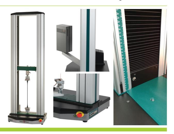
The model 25ST Extended height and speed range is a variation of the Tinius Olsen 25ST Electromechanical Materials Testing Machine. It is a robust design for use in a range of materials testing.
