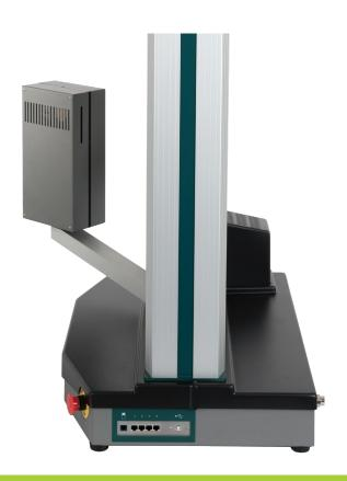
The 50ST Extended height model is a variation of the Tinius Olsen 50ST Electromechanical Materials Testing Machine. It is a robust design for use in a range of materials testing.
