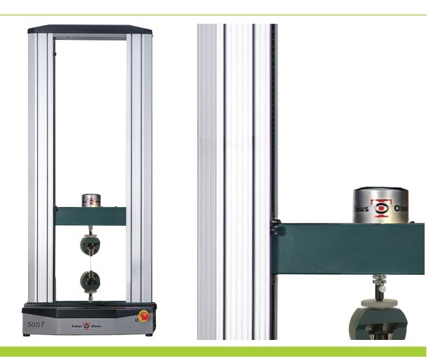
The 50ST Loadcell above crosshead model is a variation of the Tinius Olsen 50ST Electromechanical Materials Testing Machine. It is a robust design for use in a range of materials testing.
