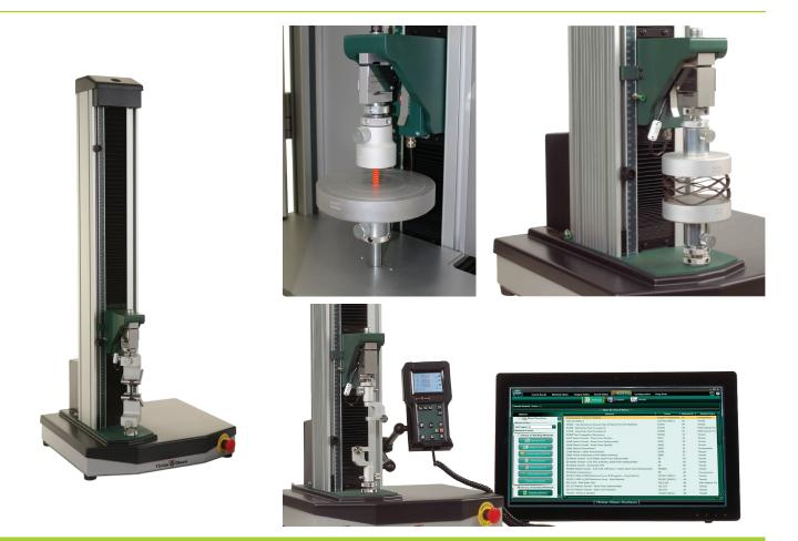
The 5ST dust & particle ingression resistance model is an Electromechanical Materials Testing Machine. It is a robust design for use in a range of materials testing.
